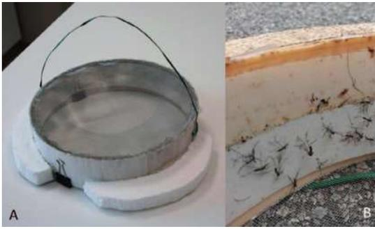
Fig. 1. Image of the (A) floating system and (B) detail of the sticky surface with adult mosquito.
